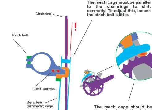
The mech cage should be positioned as close to the chainrings as possible (vertically), which means 2-5mm, or the thickness of a penny to a pound coin.
