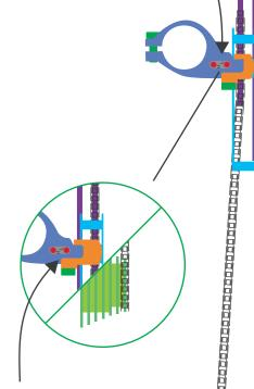
If you do have to make changes to your front limit screws, make sure you check alignment and shifting at both extremes of your gear range.
