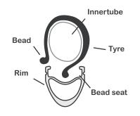
Pump the tyre to under 10psi and visually inspect the tyre to make sure it is seated evenly on the rim - check both sides! Tyres often have a seam-line in the rubber which makes it easy to check that the tyre is evenly seated.
