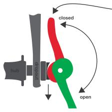
Most wheels have a quick release skewer: to remove it, open the cam lever. You may need to loosen the nut on the other side of the wheel (by turning the open cam lever counter-clockwise). With a back wheel, it helps to shift to the smallest sprocket.
