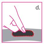
c. Peel foil backing off patch. d. Press patch firmly onto tube, then remove plastic backing.
